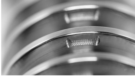
Figure 2. Artificial breakout damage on the worm.
