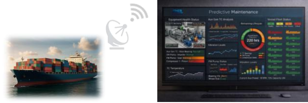
Figure 1. System data flow: Only health indicators are transmitted from the ship to the onshore Predictive Maintenance Platform via the vessel's internet connection.
