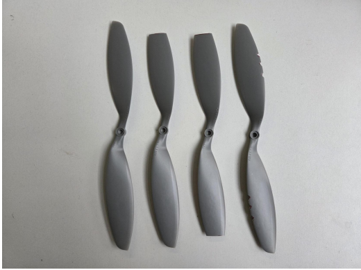
Figure 2. Depiction of damage types: no fault, one broken tip, two broken tips, notches at the leading edge of both blades (from left to right).
