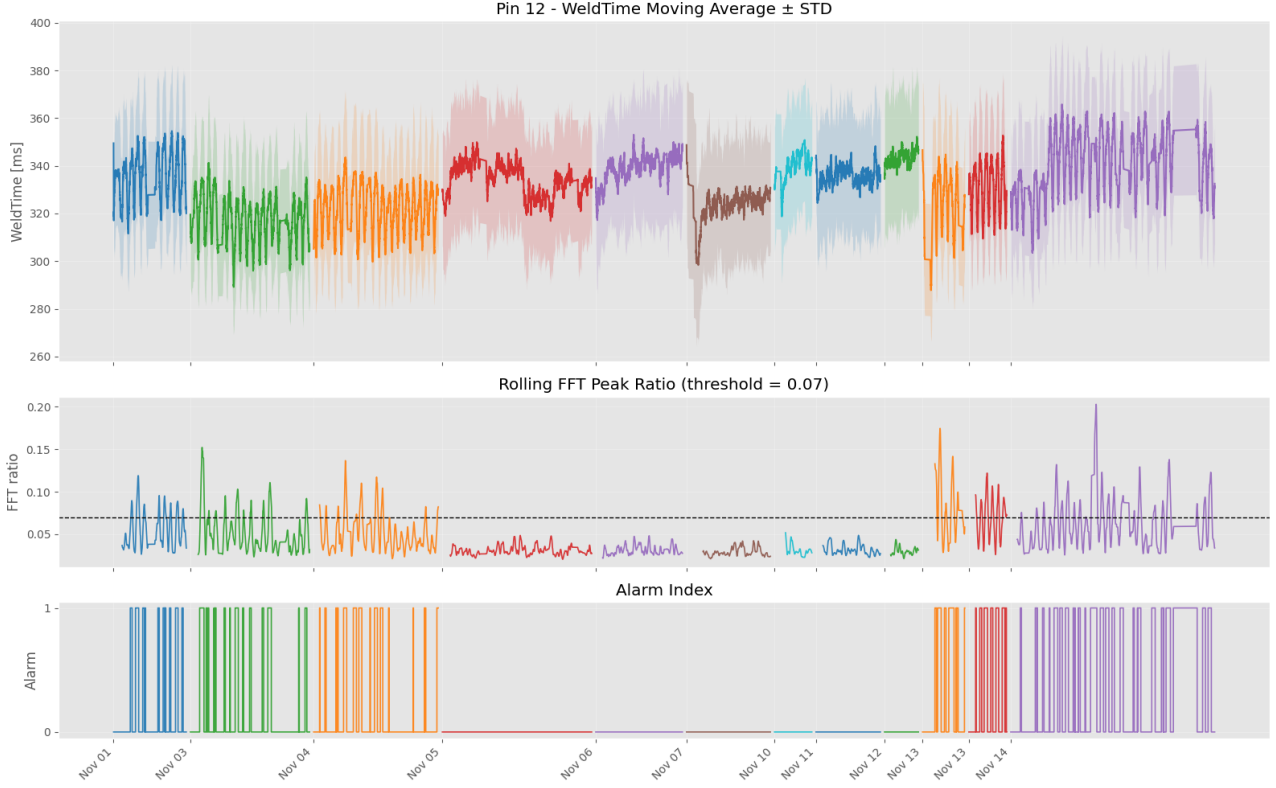
Figure 4. Results of the FFT peak ratio for detecting abnormal oscillatory behavior, along with the resulting threshold-based alarm. Each color represents a different working shift.
