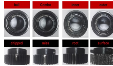
Figure 3. Gear and bearing defects.
