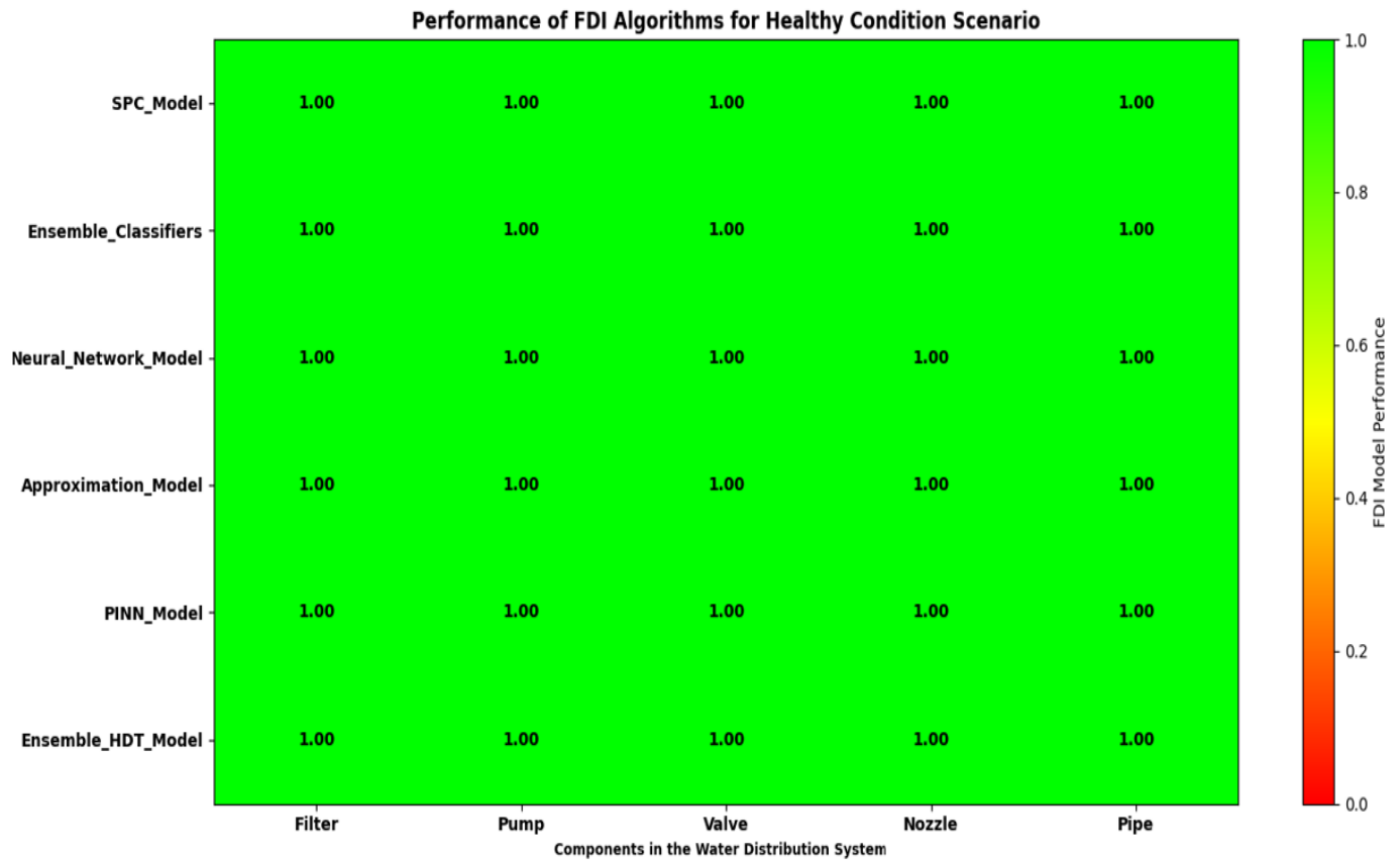
Figure 9. Performance of FDI algorithms for a Healthy Condition scenario at a pump speed of 700rpm.
