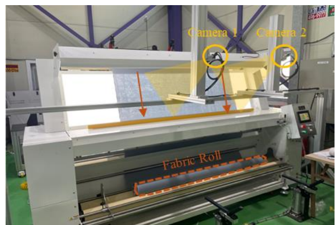
Figure 2. Image data collection using fabric inspection machine
