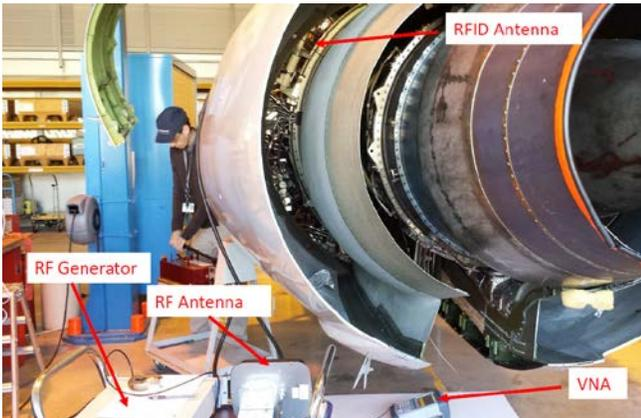
Figure 19. System tests in application environment for the first test
