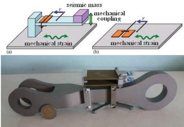
Figure 15. Kind of coupling: (a) seismic; (b) direct and real harvester
