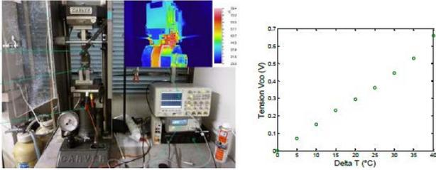
Figure 18. Thermal harvester characterization
