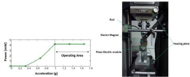
Figure 16. Vibration harvester characterization
