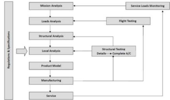
Figure 3. Fatigue and damage management
