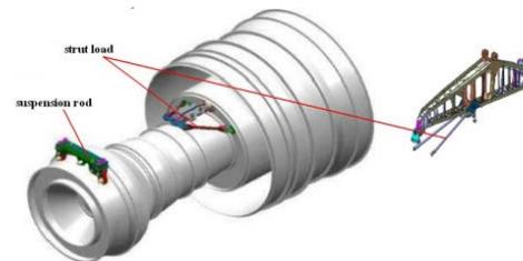
Figure 1. Engine Mounts System overview
