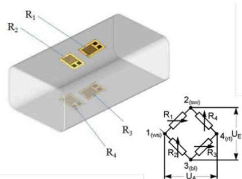
Figure 4. Strain gauge bridge
