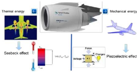
Figure 5. Energy sources in engine environment
