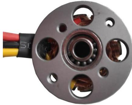
Figure 5. Motor with broken bearing cage.
