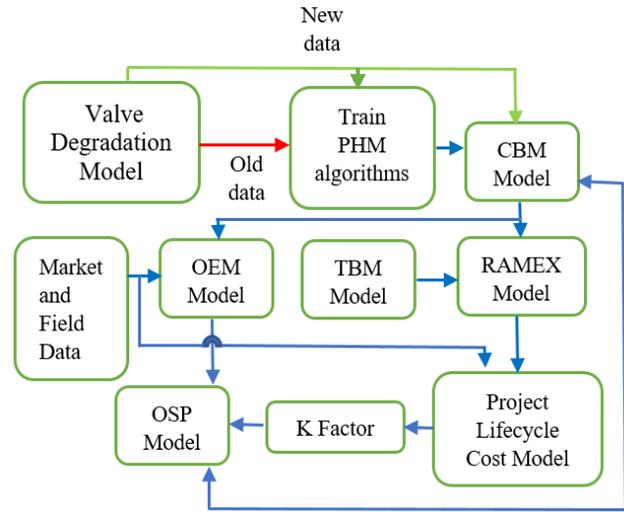
Figure 3: Block Diagram for determining OSP
