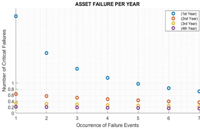
Figure 6: Number of failure of the valve that occur.
