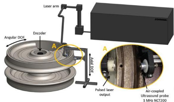
Figure 7. The laser-ultrasonic experimental set-up (Cavuto et al., 2016)
