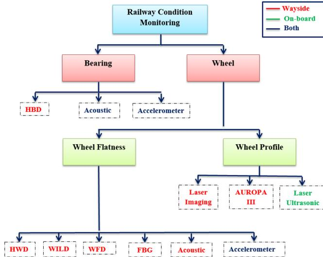
Figure 14. Overview of available CM technologies for railway bearing and wheel health monitoring
