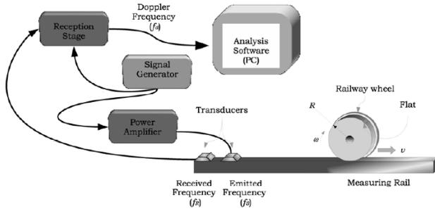
Figure 12. Wheel flat detector prototype (Brizuela et al., 2010)
