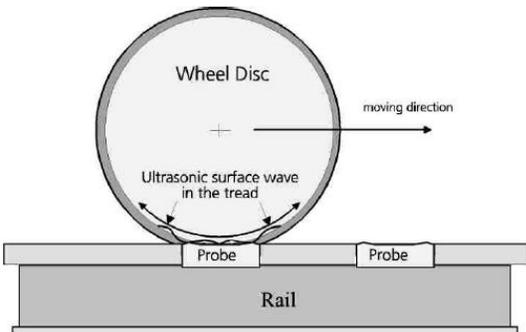
Figure 8. In-motion wheel inspection principle (Salzburger et al., 2009)
