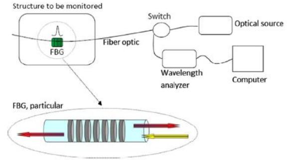
Figure 10. Schematic of the FBG sensor (Roveri et al., 2015)
