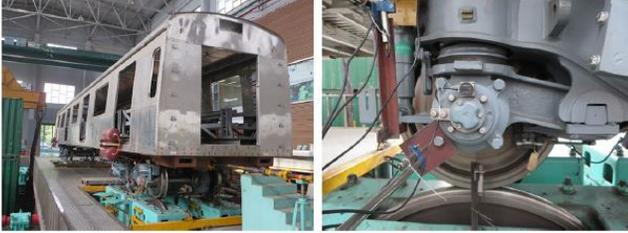
Figure 9. Rolling stock simulator (Li et al., 2016)
