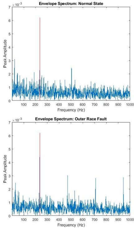
Figure 12. Comparison of bearing conditions at time-step 5 vs time-step 600
