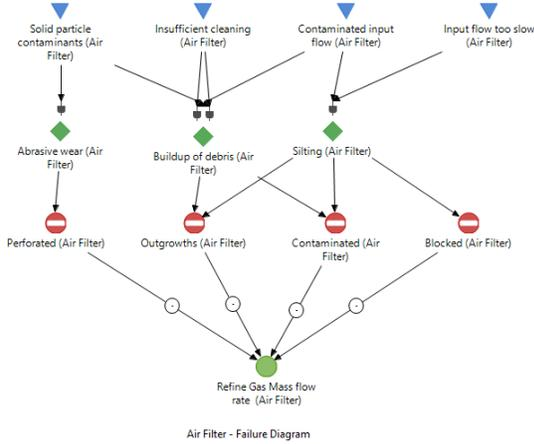
Figure 4. Failure diagram
