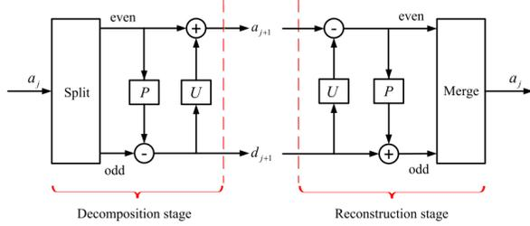
Figure 7. Lifting scheme (Liu et al., 2017)
