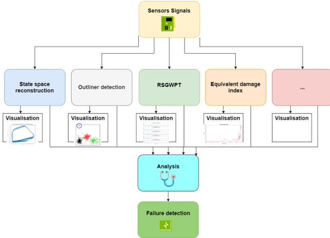
Figure 10. Failure identification techniques
