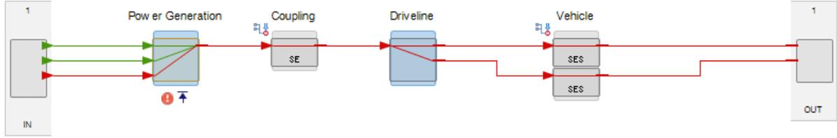
Figure 3. System model of a vehicle system
