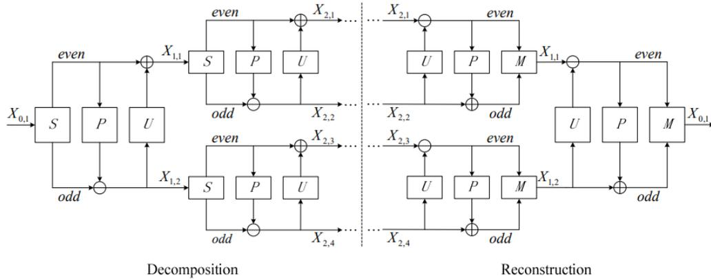
Figure 8. SGWPT Lifting scheme (Tong et al., 2017)
