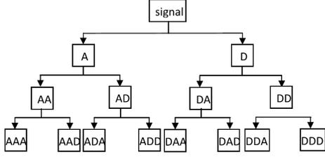
Figure 6. Wavelet packaged transform decomposition (Loutas & Kostopoulos, 2012)
