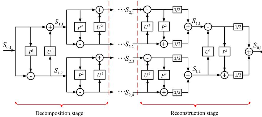
Figure 9. Redundant Lifting scheme (Liu et al., 2017)
