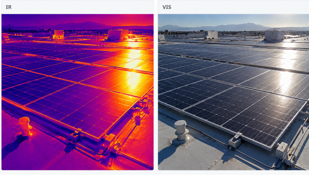
Figure 1. The “phantom fire” pattern motivating this paper. Left: long-wave IR image of a solar-panel array showing a bright, high-temperature region (false alert). Right: the paired visible image of the same scene at the same instant, in which the bright region is plainly the sun specularly reflected off the panel surface — not a thermal anomaly. Without a visible-modality check, the IR pixel-threshold rule cannot distinguish these two cases.
