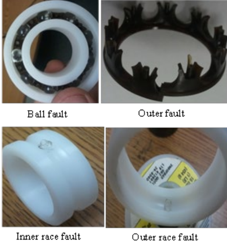
Figure 4. The 4 seeded bearing faults used in the tests: inner race fault, outer race fault, ball fault, and cage fault.
