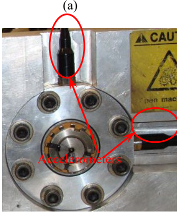
Figure 5. The layout of the two accelerometers, screw-mounted on the bearing housing in the bearing test rig.
