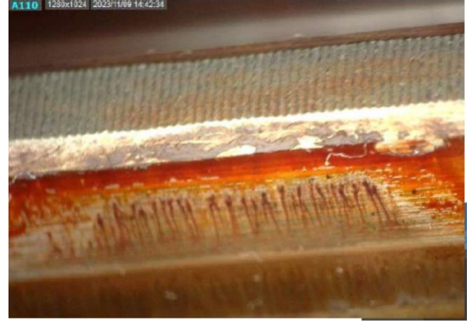
Figure 1 Scuffed Gear in Industrial Compressor
