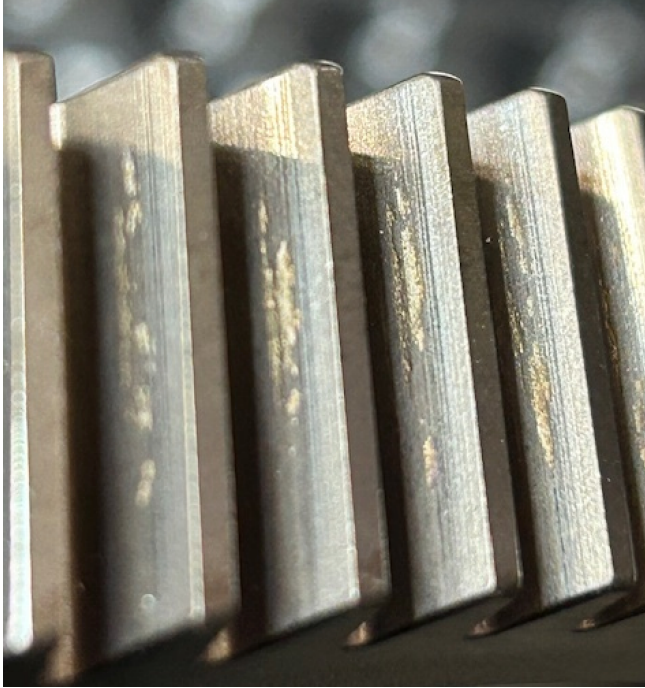
Figure 1 Wear found on the N2 Pinion
