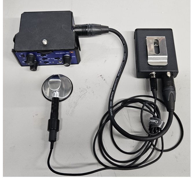
Figure 2. Custom stethoscope used in the experiment, including audio pre-amp, audio amplifier, digital microphone, and stethoscope.
