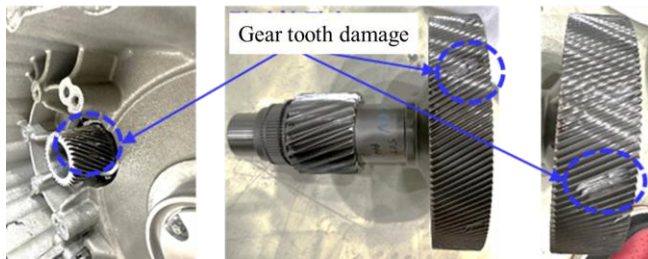
Figure 24. Disassemble and check for faulty parts
