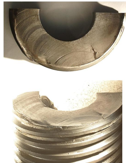
Figure 3. Optical fractographic photos of the fracture surface of the failed driveshaft. Evident beach marks with the single origin at the root of the last engaged thread were revealed. The fracture surface was relatively flat with one ratchet mark present next to the fatigue origin.
