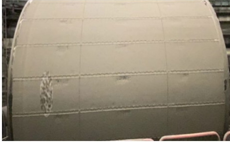
Figure 19. Synthetically generated cloth failure resembling texture irregularities.
