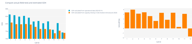
Figure 16. Results from field validation scenario 6. Estimation from operational data underestimated SOH in all cells. Almost 1 year storage of module between ECM based SOH calculation and lab capacity checkup.
