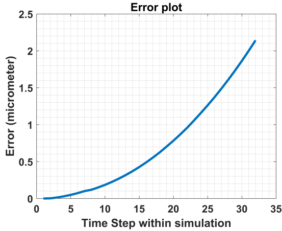
Figure 7. Error Between Predicted and Actual Flank Wear for Set Threshold of 0.05 \mu m .
