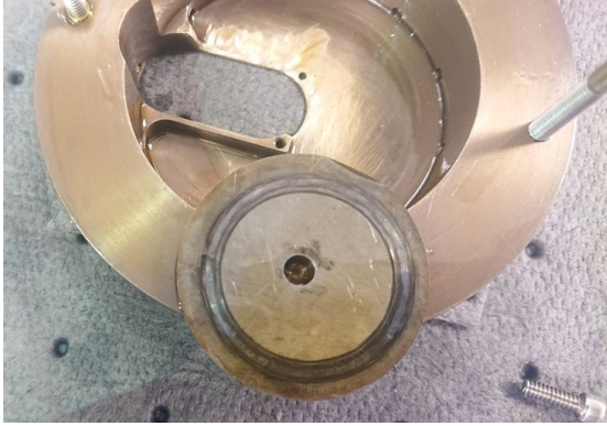
Figure 23. SAE 9310 carburized steel disk after test.
