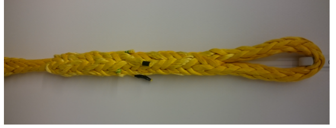
Figure 2. Example of splice and eyelet at the end of a fiber rope specimen.
