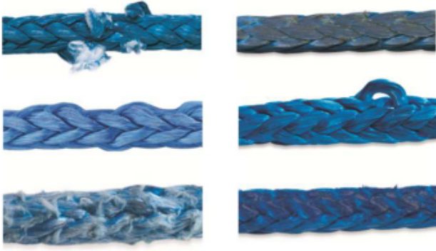
Figure 1. Different kinds of rope damages. Cut strands (top left), compression damage (top right), inconsistent diameter (middle left) and pulled strands (middle right), heavy abrasion (bottom left) and melted fibers (bottom right). Reproduced with permission from Samson Rope Technologies.
