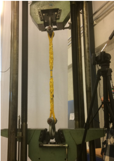
Figure 4. Experimental set up. Here a fiber rope is secured into the tensiometer.
