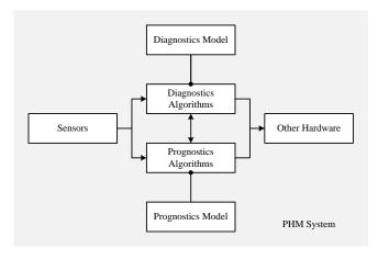
Figure 1. Typical components of a PHM System.
