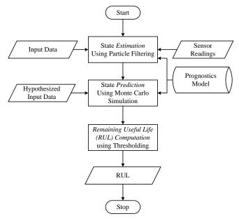
Figure 2. Flowchart of ComputeRUL, an example prognostics algorithm.
