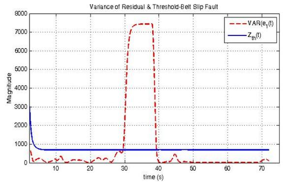
Figure 9. Residual of  $S_1$  signal for belt slip fault.
