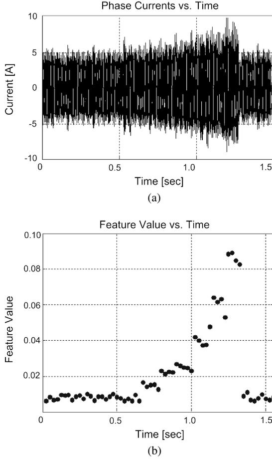
Figure 8: Plot of (a) three-phase current data and (b) features computed from experimental data.
