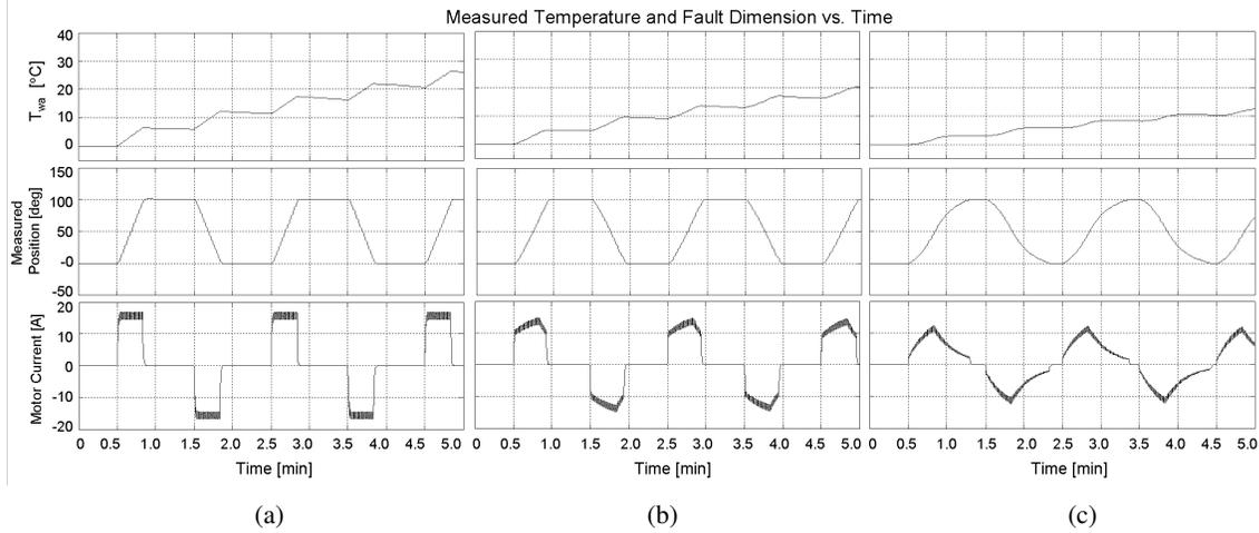
Figure 16: Simulation results for the reconfigurable control with initial fault dimensions (a)  $L_0 = 1 \times 10^{-6}$  (b)  $L_0 = 1 \times 10^{-2}$  and (c)  $L_0 = 1 \times 10^{-1}$
