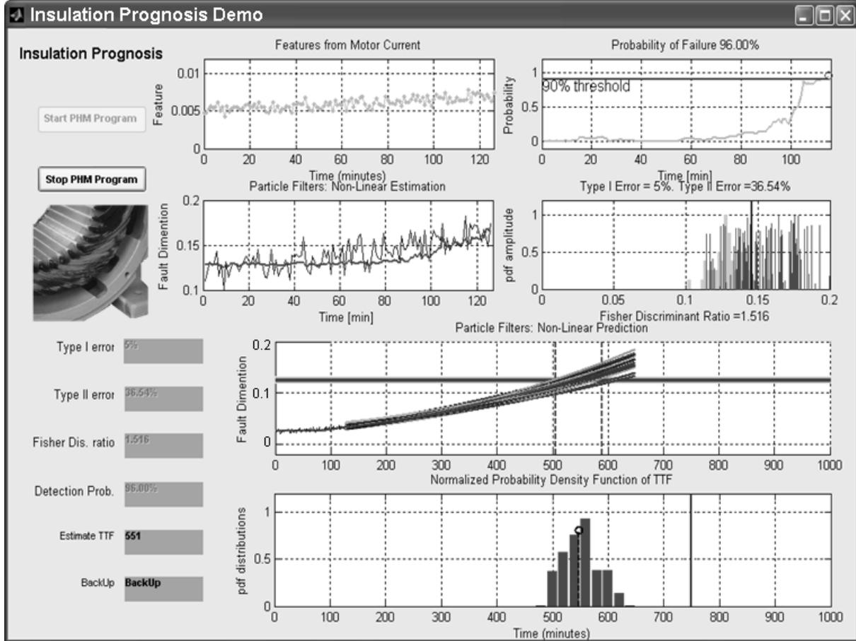
Figure 11: Example of particle filter based prognosis using artificial data.
