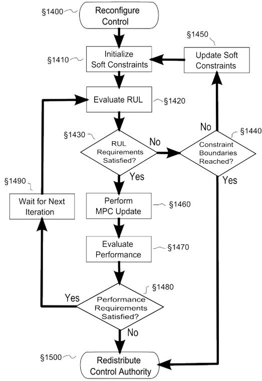
Figure 5: Flowchart of the reconfiguration state.
