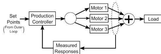
Figure 2: Block diagram of the triplex redundant EMA.
