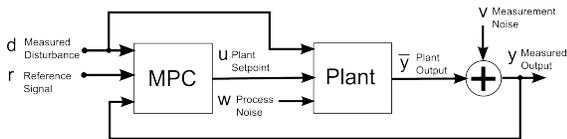
Figure 14: Block diagram of MPC with plant and signals
