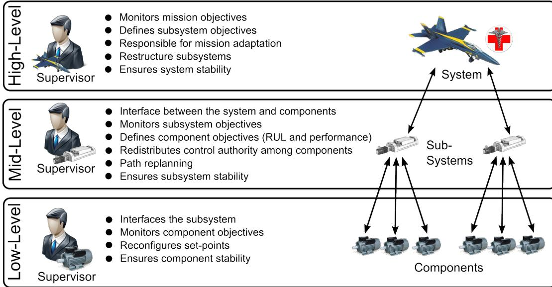
Figure 3: Reconfigurable control architecture 3-tier hierarchical strategy.
