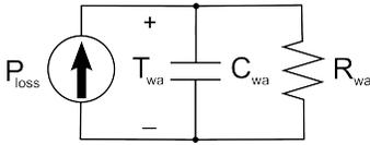
Figure 10: Schematic of the simplified thermal model.
