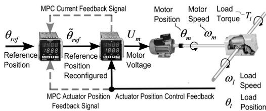
Figure 12: Block diagram showing actuator inputs and outputs
