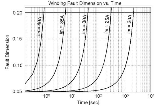
Figure 15: Fault dimension trajectories for different current values.
