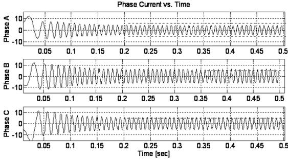
Figure 6: Simulation illustrating phase current asymmetry.
