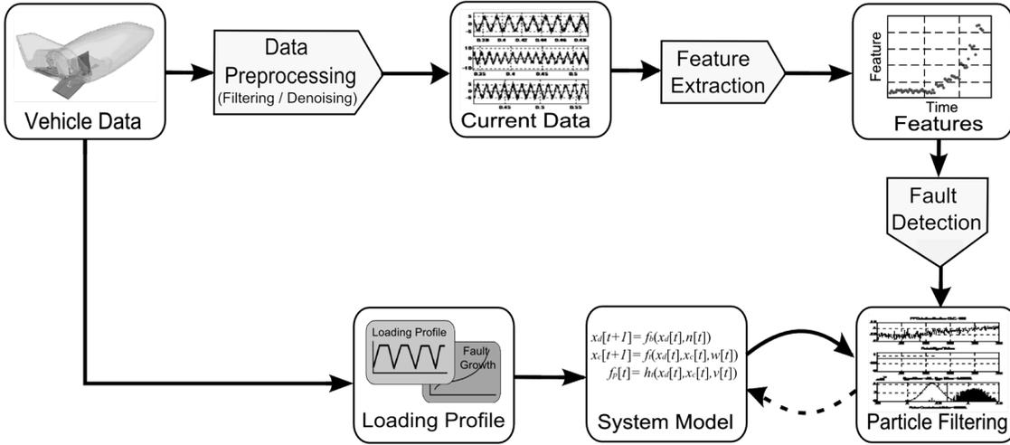
Figure 7: Particle filter-based fault detection architecture.
