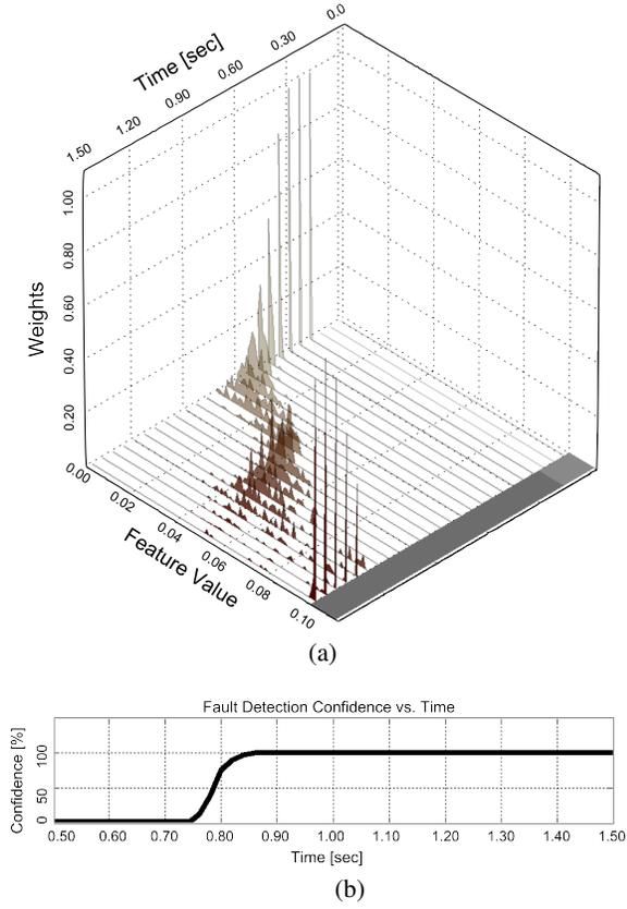
Figure 9: Fault detection using experimental data. Illustrated are (a) the results after applying a particle filter to the incoming feature and (b) the level of confidence computed from the particle weights.
