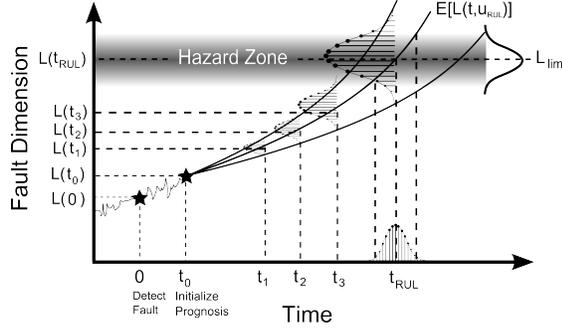
Figure 13: Prognosis prediction of fault dimension highlighting the control input corresponding to the targeted RUL.
