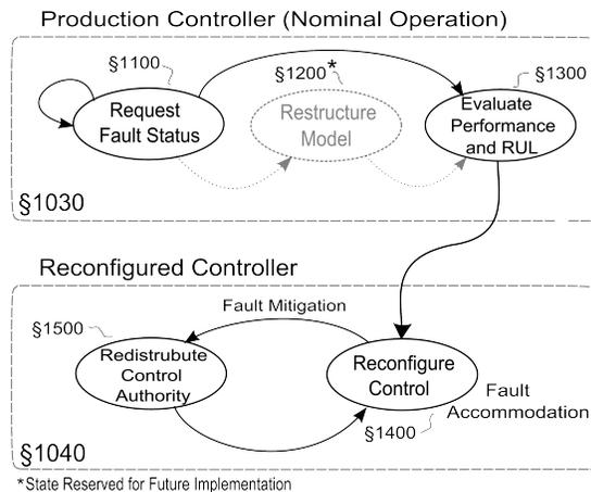
Figure 4: State transition diagram for low-level reconfigurable control.
