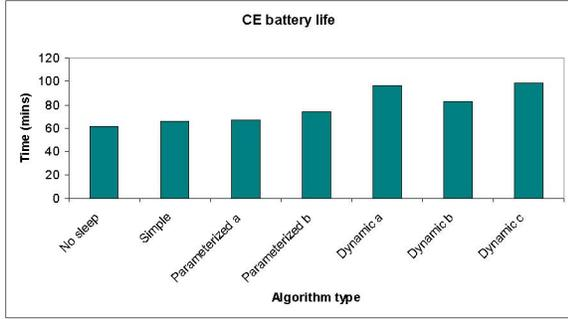
Figure 9: Battery life with different power management schemes compared with no power management scheme.
