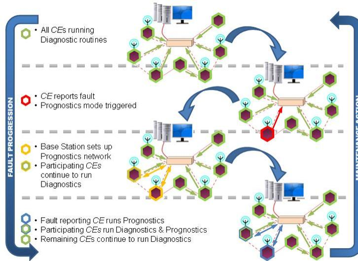
Figure 2: Flow diagram for diagnostics and prognostics operations in the distributed architecture. (Adapted from figure 2 in (Saha *et al.*, 2009).
