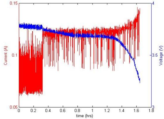
Figure 10: Current and discharge profile for CE with no power management schemes.
