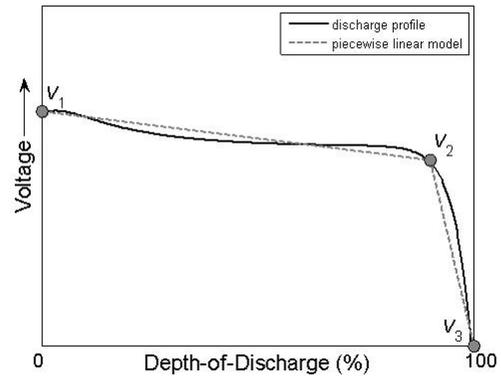
Figure 4: Typical discharge curve of a Sun SPOT Li-ion battery with piecewise linear model fit.
