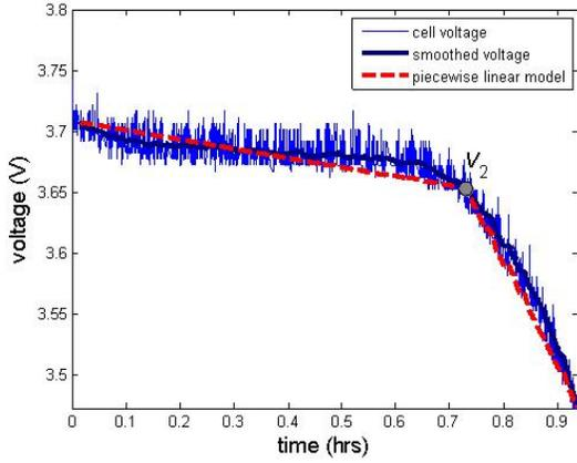
Figure 5: Model identification from a specific discharge cycle.
