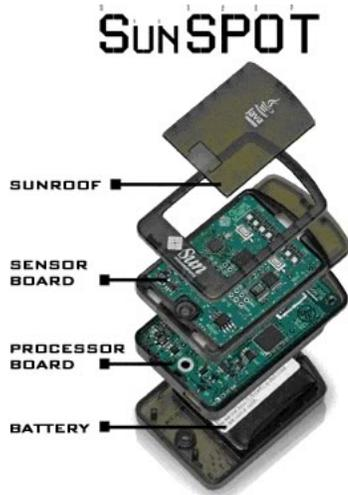
Figure 3: Anatomy of a free ranging Sun SPOT device (courtesy of [www.sunspotworld.com](http://www.sunspotworld.com)).
