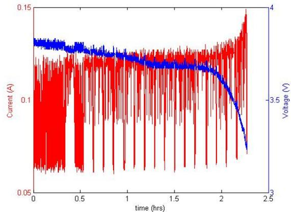
Figure 11: Current and discharge profile for CE with *dynamic* power management schemes with varying  $f_{diag}$ . The dip in current values correspond to sleep states.
