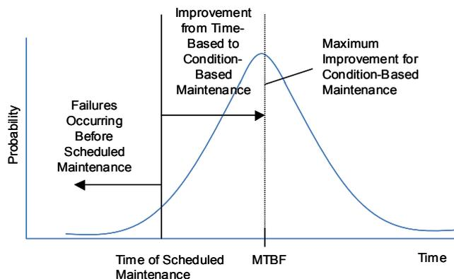
Figure 1. Extending Life by Transitioning to Condition-Based Maintenance.
