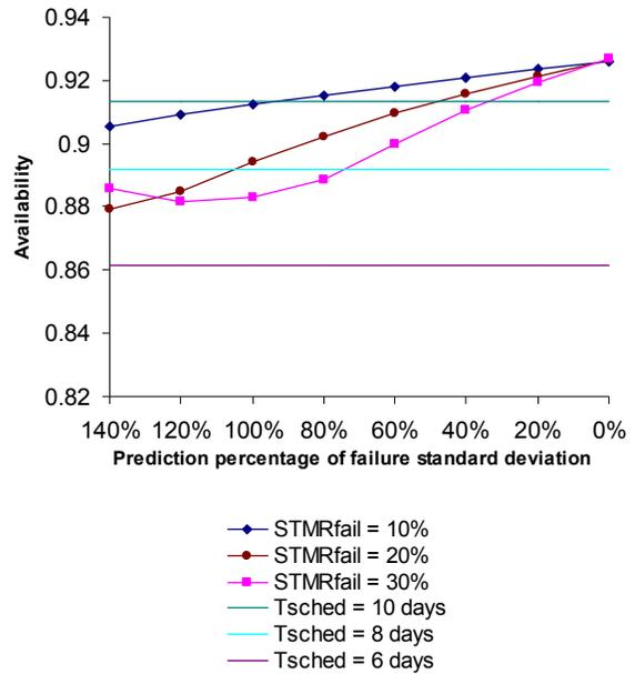
Figure 7. Availability for varying prediction percentage of failure standard deviation by  $STMR_{fail}$ .
