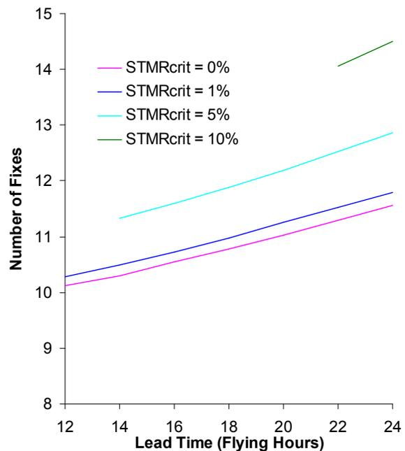
Figure 6. Number of fixes for varying prediction precision ( $STMR_{pred}$ ) by lead time for  $STMR_{crit}$  of 10%.
