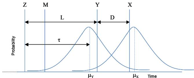
Figure 4. Model relating PHM events (time of prediction Z and predicted time of failure Y), failure event (X), maintenance opportunity (M), and times between them.
