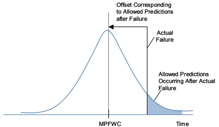
Figure 3. MPFWC is fixed relative to actual failure by allowed predictions occurring after actual failure (or *false negatives*).
