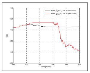
Figure 5: RSPF-based parameter estimate,  $\delta$ = {0.05, 0.15}
