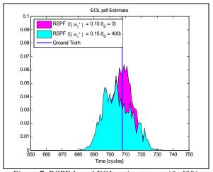
Figure 7: RSPF-based EOL estimate,  $t_0 = \{0, 400\}$
