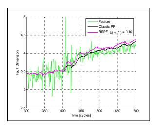
Figure 2: RSPF-based state estimation,  $E\{\omega_1^*\}=0.10$
