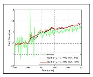
Figure 4: RSPF-based state estimation,  $\delta = 0.05$  vs.  $\delta = 0.15$
