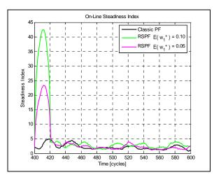
Figure 10: RSPF-based prognostic algorithm. RUL-OSI (steadiness) index
