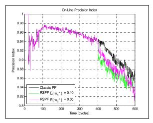
Figure 8: RSPF-based prognostic algorithm. RUL-OPI index
