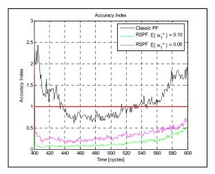
Figure 9: RSPF-based prognostic algorithm. RUL accuracy-precision index
