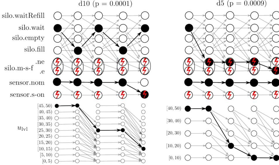
Figure 5: The inferred system trajectories (black filled circles and arrows) for the sensor-fault scenario as trellis diagram for d10 for  $u_{1vl}$  (left) and for d5 (right). Grey shaded arrows show possible transitions (probability  $> 0$ ).
