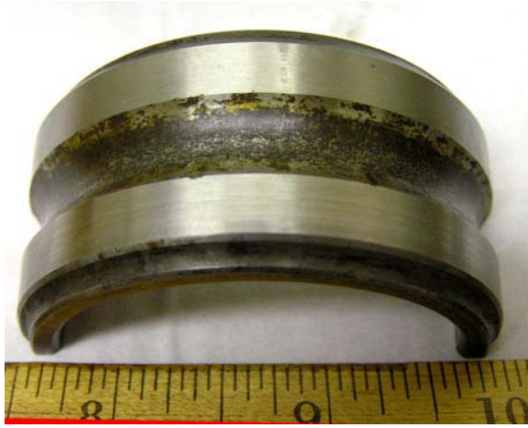
Figure 2. Inner Race Showing Defects
