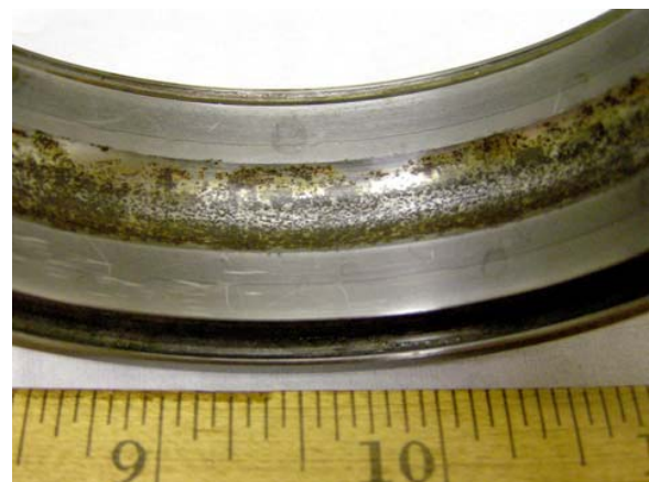
Figure 1. Outer Race Showing Damage
