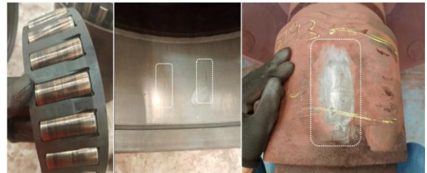
Figure 6. Wagon 1, bearing 1, right side, with nonconformity marks on rollers and cup.
