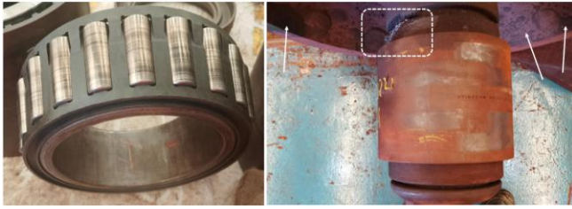
Figure 7. Wagon 2, bearing 3, right side, with nonconformity marks on rollers and signs of grease leakage.
