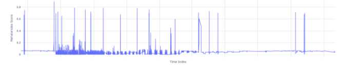
Figure 13: Mahalanobis score for actuator_2_pressure on "DELTA"
