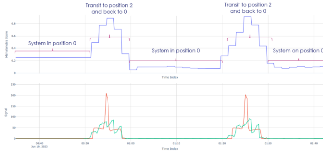
Figure 11: Mahalanobis spikes analysis on June 19, 2023 on "Delta" radar
