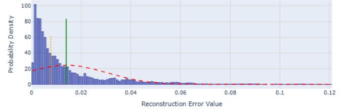
Figure 4: Reconstruction errors distribution for actuator_1_pressure
