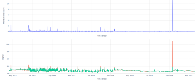
Figure 19: Mahalanobis score and reconstructed signal for oil_tank_temperature
