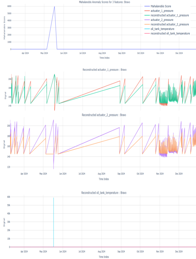
Figure 26: Mahalanobis score, signals and all reconstructed signals for "BRAVO"
