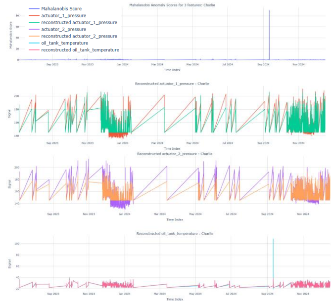
Figure 23: Mahalanobis score, signals and all reconstructed signals for "CHARLIE"
