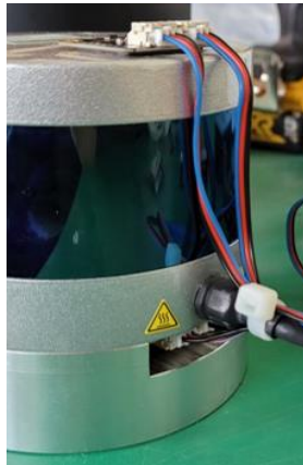
Figure 3. LIDAR with additional sensors.
