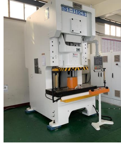
Figure 1. A single-point direct drive servo press (Chin Fong Machine Industrial Co., Ltd, 2023)
