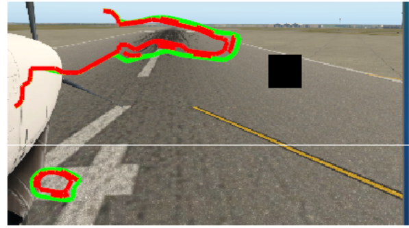
Figure 9. ACT camera image with "dirt" spot (black rectangle) and superimposed boundary lines for high risk regions
