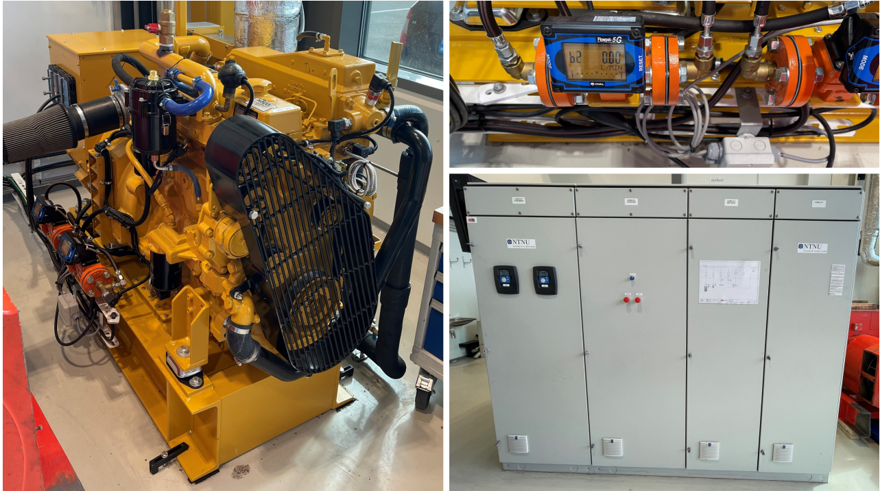
Figure 4. Test bench: Marine diesel engine, sensors and power switchboard
