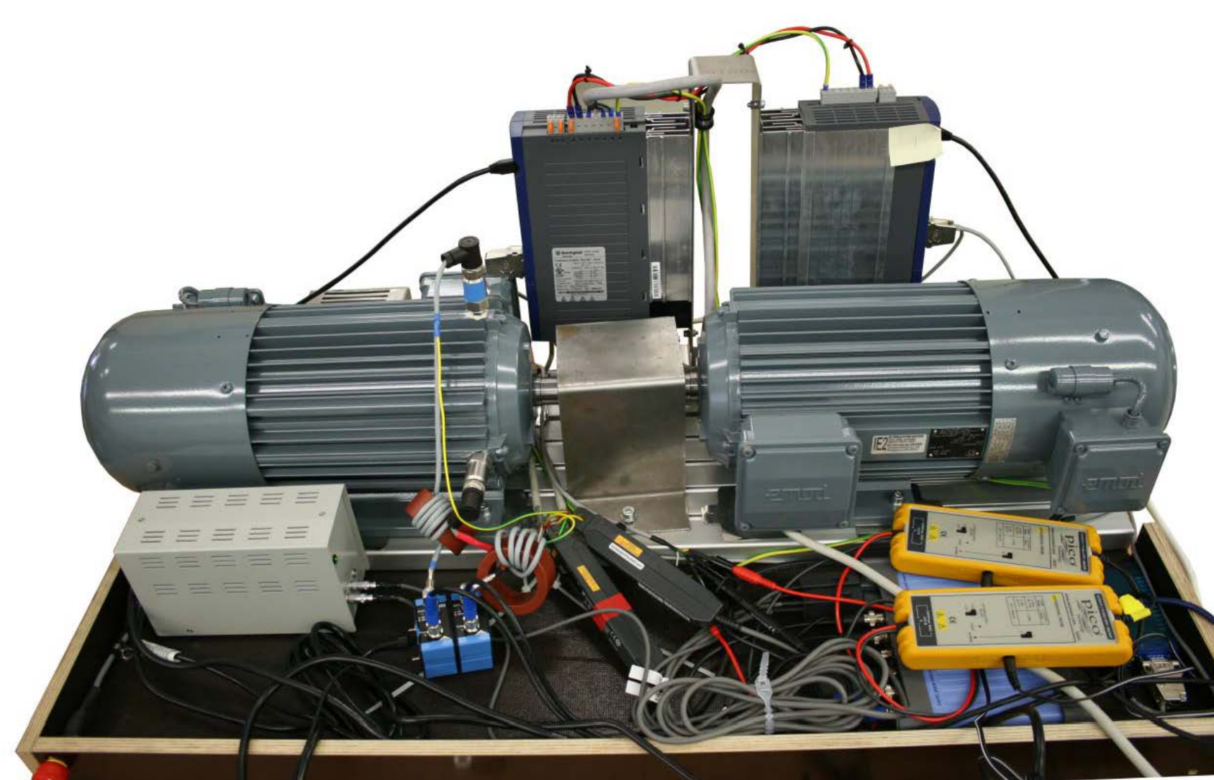
Test bench (model: EMOD FKFIE2100LA, Pmech: 3 kW, nnom: 1440 /min, Vnom: 400V, Inom: 6.4A, cosφ: 0.78)
