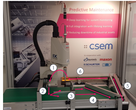
Figure 1. Structure and steps of the quality control pipeline for electrical fuses (PHM Society, 2021)
