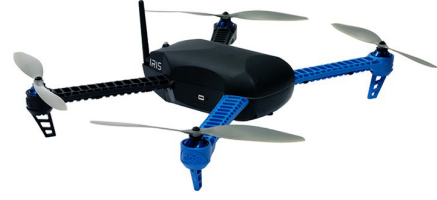
Figure 4. Multi-rotor platform used for validation. 3DR IRIS+ Quadcopter.
