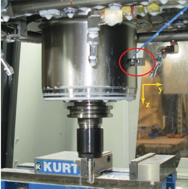
Figure 3. Picture of the magnetically mounted tri-axial accelerometer (circled in red) on the CNC spindle housing with the direction of its positive y and z-axes.
