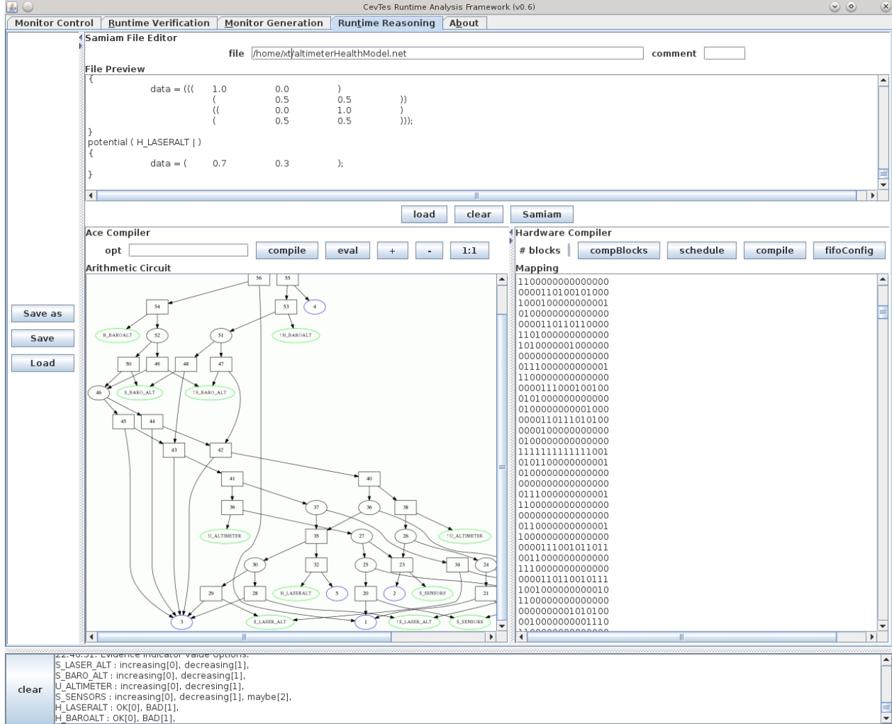
Figure 6. Screenshot of our GUI-based BN synthesis tool. There is a textual description of the altimeter health model Bayesian network (top), a compiled arithmetic circuit of the network (bottom left), and a binary configuration for our \mu Bayes unit (bottom right).
