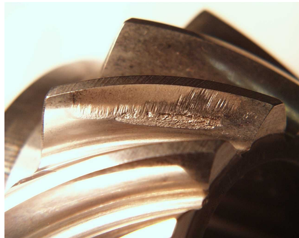
Figure 3 Pitting Damage on EX4
