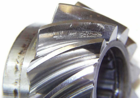
Figure 5 Damage on Gear EX5
