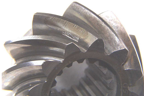
Figure 7 Damage on Gear EX6
