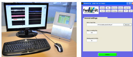
Figure 9. (left) Labview VI for raw signal visualization and (right) the graphical user interface to set the optional parameters (if required) of the signal processing algorithms.
