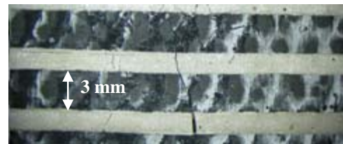
Figure 3: Photograph under microscope of impacted region of FFRP laminate. Painted silver electrodes are 1.5 mm wide and spaced 3 mm edge-to-edge.
