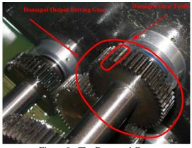
Figure 9: The Damaged Gear
