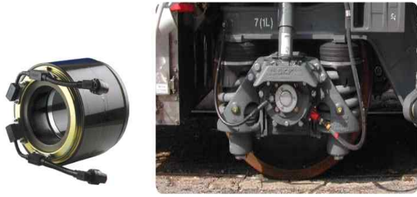
<Fig. 3 Application of Axle Bearing Sensor Developed by SKF>
