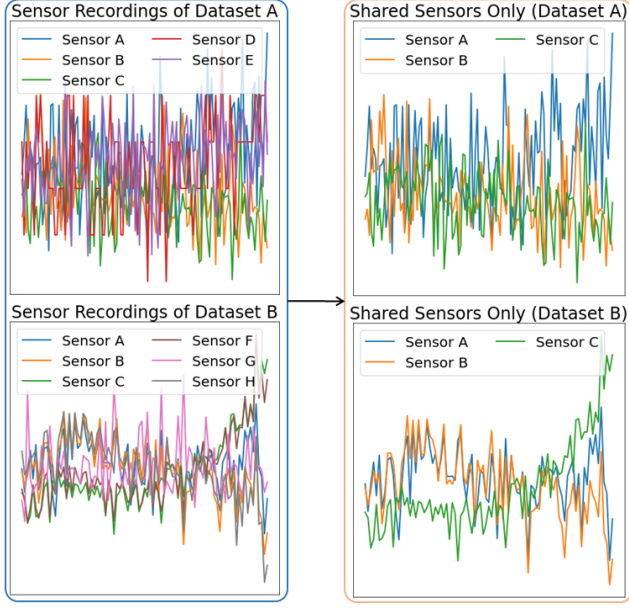
Figure 3. Feature alignment based on shared sensor intersection across different datasets.
