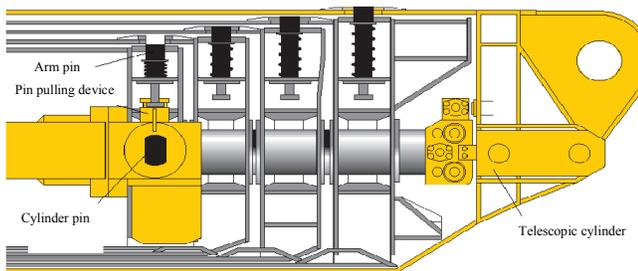
Figure 3. The schematic diagram of the crane single cylinder latch telescopic arm
