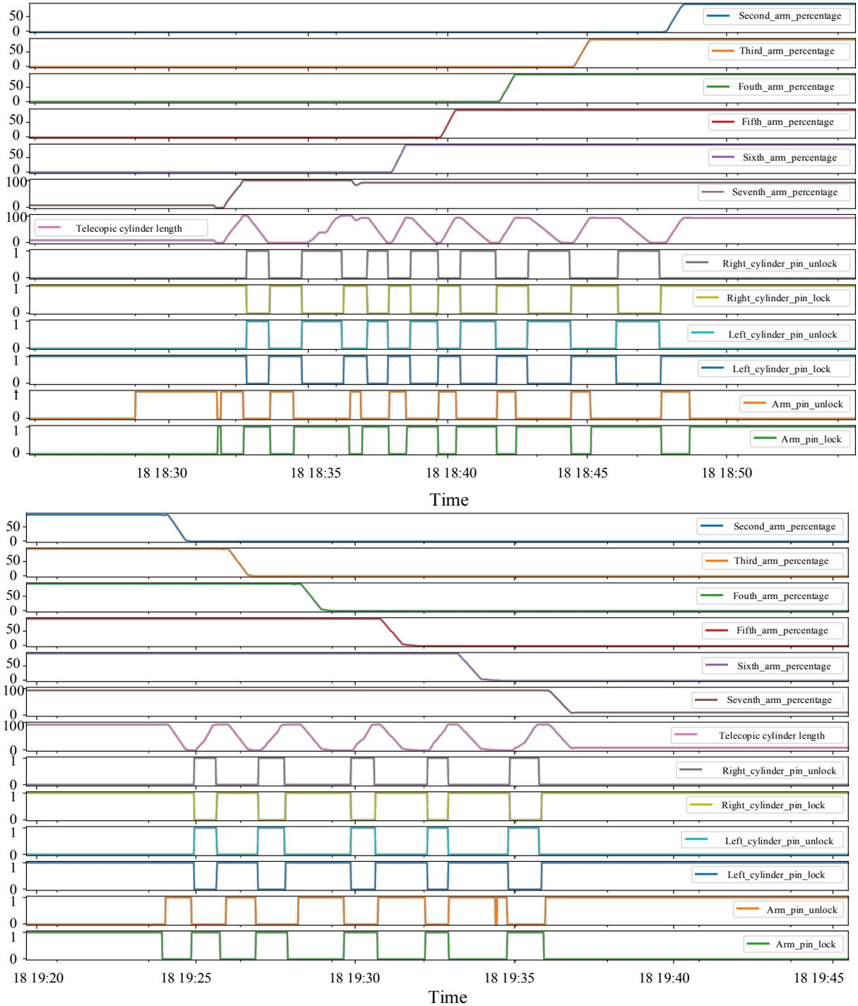
Figure 4. The arm extension process and the arm contraction process
