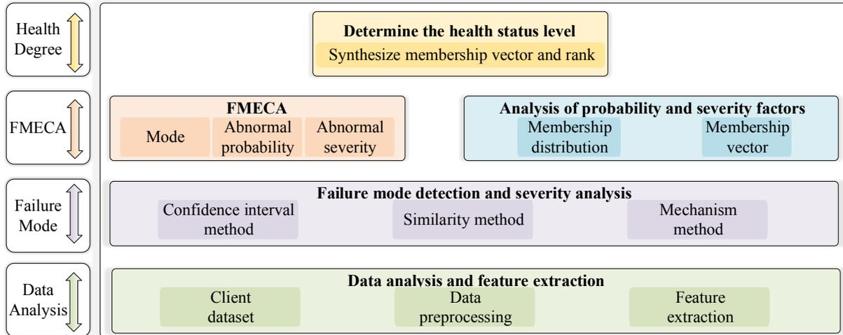
Figure 2. Device health assessment based on FMECA
